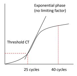
The number of cycles the PCR takes to reach a set threshold is known as the CT value. This is inversely correlated to the amount of template DNA in the sample.
